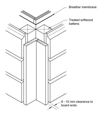
Figure 5.41 Re-entrant corner in horizontal boarding
