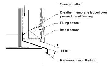
Figure 5.28 Vertical boards over flashing
