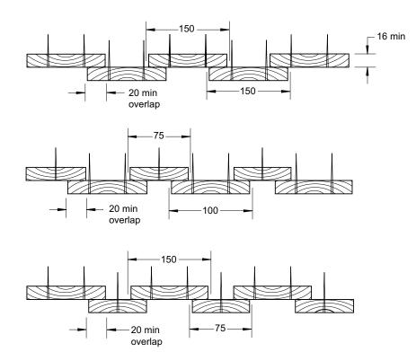
Figure 5.18 Profiles suitable for vertical boarding
